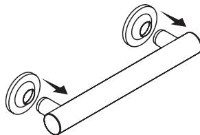
**7.** Slide escutcheons over wall plates. Secure the grab bar in place with the setscrews provided.
